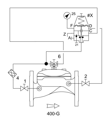
Suitable build for 400 series valves from 6" up to 12" for irrigation applications
