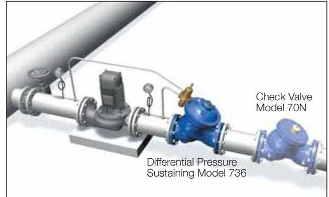
Where suction pressure regimes vary, the Model 736 is needed to limit pump flow by sustaining pump differential pressure, preventing pump overload and cavitation damage caused by excessive demand.
