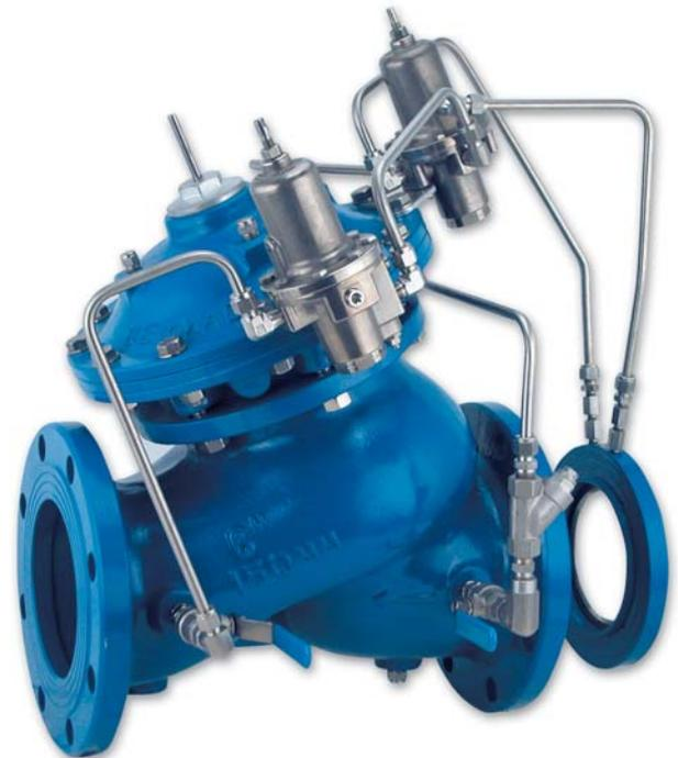
The Model 772-U Flow Control and Pressure Reducing Valve is a hydraulically operated, diaphragm actuated control valve with two independent functions. It maintains both pre-set maximum flow and reduces higher upstream pressure to lower constant downstream pressure, regardless of varying demand or upstream pressure.
