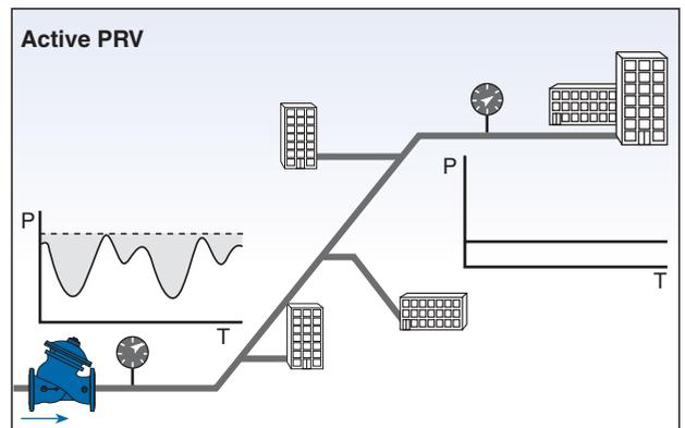
The Model 718-03 and controller continuously corrects the PRV's set value to ensure the minimum required pressure at the system critical point. As a result, the average network pressure dramatically decreases, reducing system leakage flow, burst, maintenance, energy and chemical costs.
