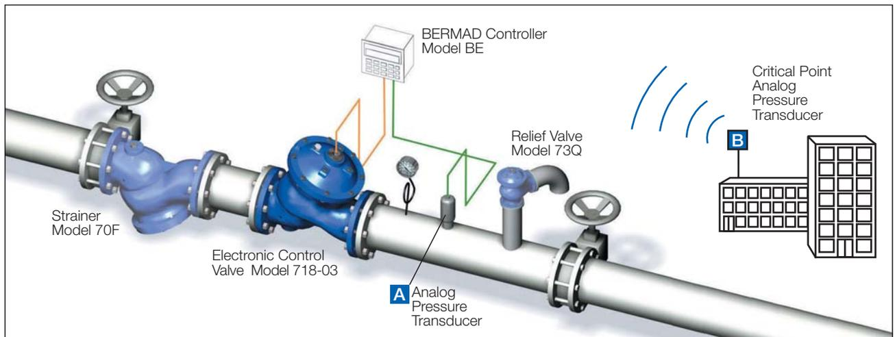
Installing the pressure transducer downstream from the valve provides a pressure reducing feature.
