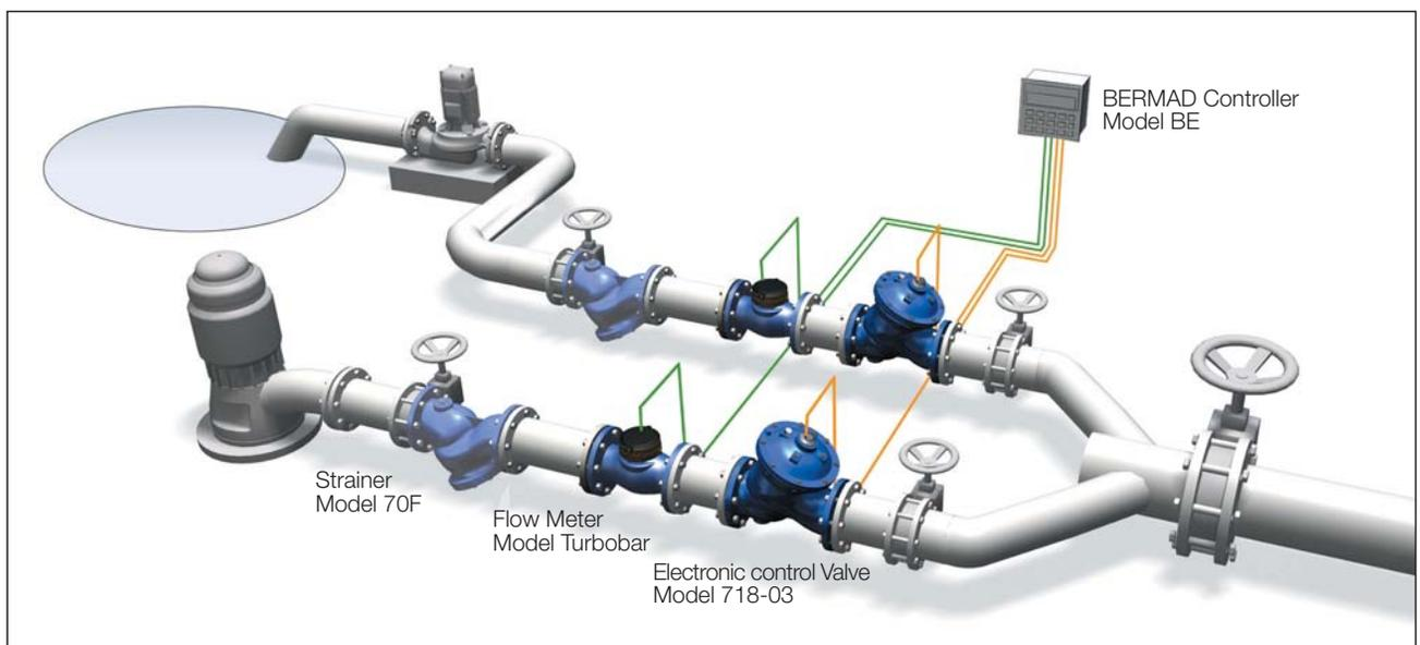
The controller receives continuous inputs from both flow transducers and corrects, in real-time, the opening of each valve, thus maintaining constant flow ratio between the two sources to achieve the desired result.
