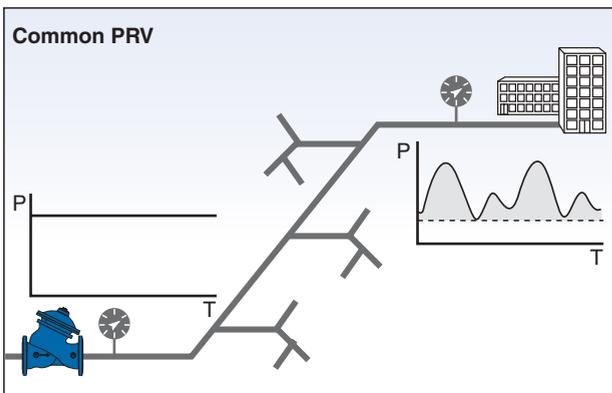
Common PRVs are set to keep the downstream pressure constant, ensuring sufficient pressure at the system critical point during "peak" demand (when line friction head loss is highest).
