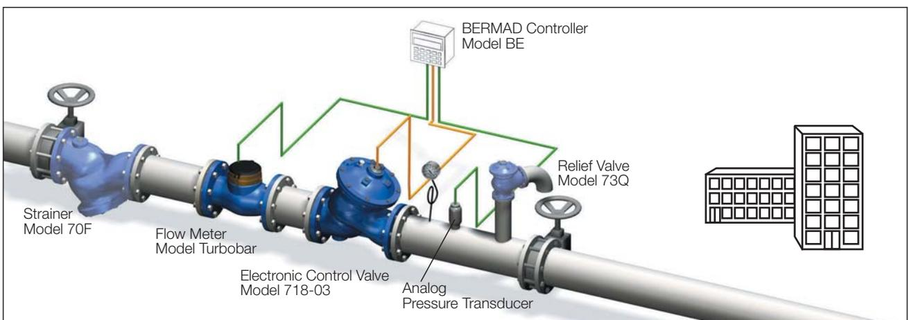
Data logging and analysis of the distribution network parameter values enable establishing a function for real time adjustment of pressure according to system demand. The flow and pressure transducers continuously transmit to the controller which reacts by adjusting the Model 718-03 according to the pre-established function.
