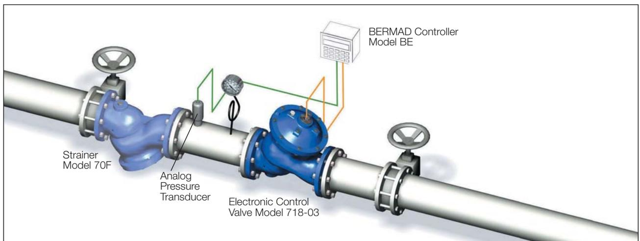
Installing the pressure transducer upstream from the valve provides a pressure sustaining feature:
