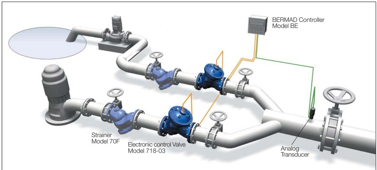
The controller receives continuous inputs from the analog transducer (conductivity, salinity, temperature etc.) and corrects, in real-time, the opening of each valve in comparison with the programmed value.
