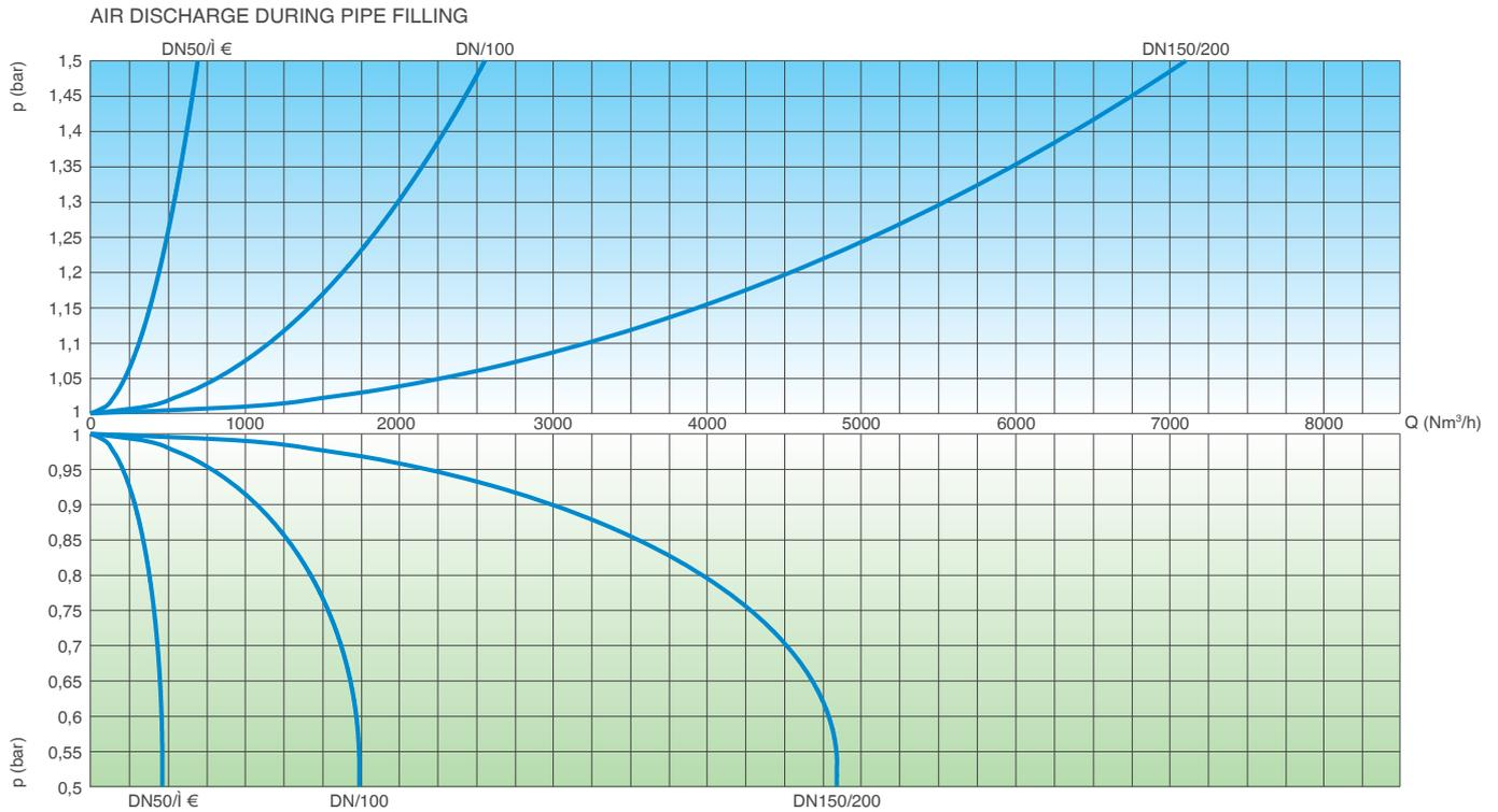
The air flow charts were created in Kg/s from laboratory tests and numerical analysis, then converted using a safety factor.
