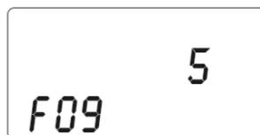
Within a specific function, the functionality of the buttons may be different (see FUNCTIONS); in this example, P4/P3 increases and decreases the value of the parameter shown on the first line, P2 confirms the value and returns when the function is selected, P1 stops the operation and returns to the main screen
