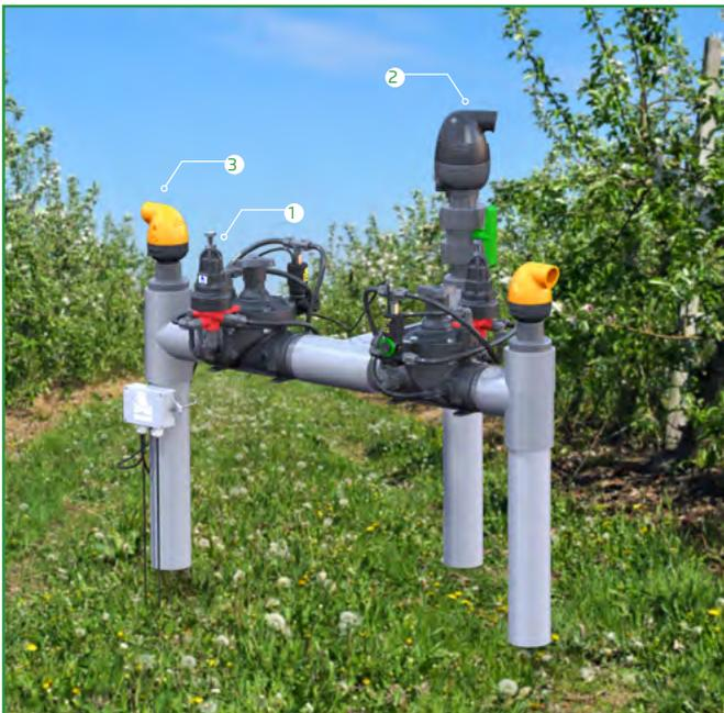
[1] BERMAD Model IR-220-55-3W-X opens in response to electric signal, and establishes reduced pressure zone protecting laterals and distribution line.
