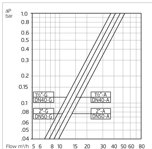
Valve flow coefficient, Kv or Cv
