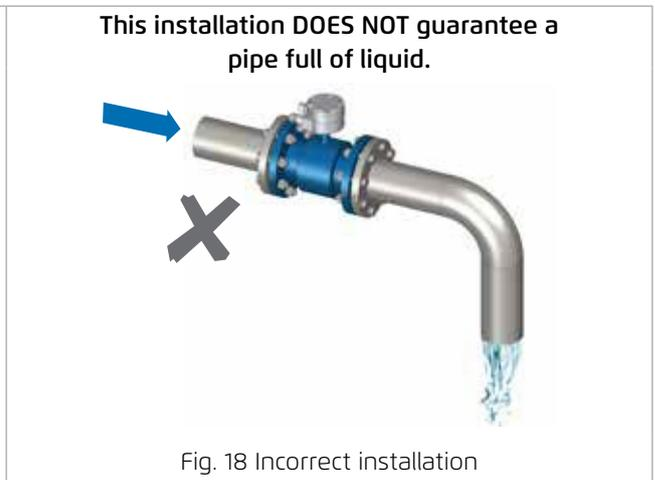
We recommend installing the sensor on a vertical/sloped pipe with an upward flow direction (Fig. 19) to minimize the wear and deposits in the sensor. Avoid the installation on vertical pipes with free exit (Fig. 20).
