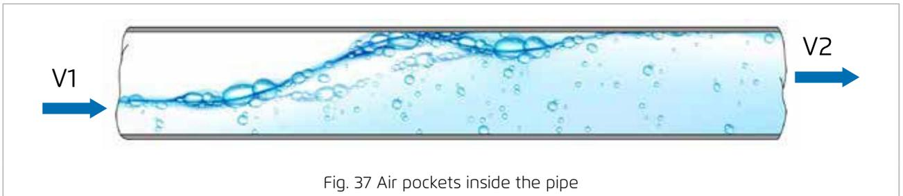
Fig. 37 Air pockets inside the pipe
