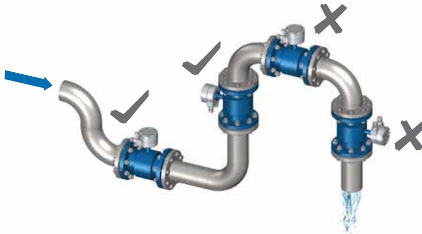
Fig. 24 Incorrect installation
