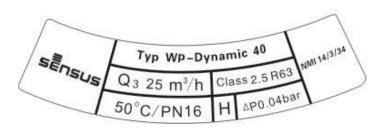
Showing Typical Markings - Note that pressure markings should be in kPa (not 'bar')
