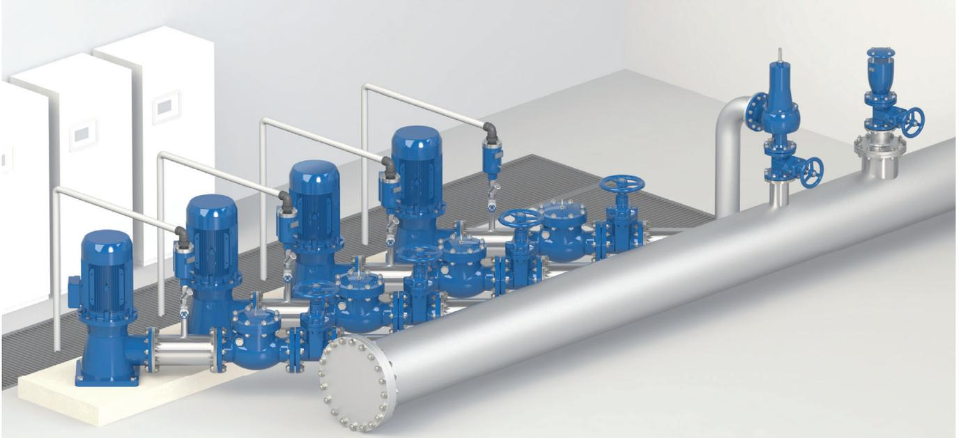
**Pressure reduction valve station.** In this second layout Gemina is installed downstream of a pressure reduction valve station to prevent in any case rise in pressure on the main line. The installation also includes the pressure reducing valve CSA XLC 310/410, a by-pass for maintenance and anti-surge combination air valves FOX or LYNX 3F AS upstream and downstream.
