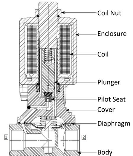
**WARNING:** This product shall be installed and wired by an authorize electrician only. The conduit hub on the enclosure must be supported against torque during assembly by using appropriate tools. While tightening a fitting into the conduit hub, attention must be paid that a max. torque of 20 Nm is not exceeded.
